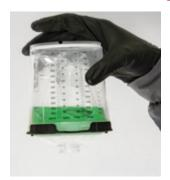
Cup B: The liner system created a major restriction, visibly showing that it would starve the spray gun of fluid. The final 8 oz. of fluid in the cup would not flow out of the cup.
