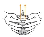
With the lid tab facing away, use forefingers to open lid. Allow paint to drain from the lid into the cup prior to opening completely.
